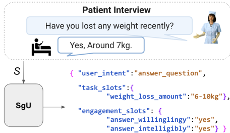
Fig. 4: Illustration of signal understanding to obtain user intent and task-related and engagement-related slots.
